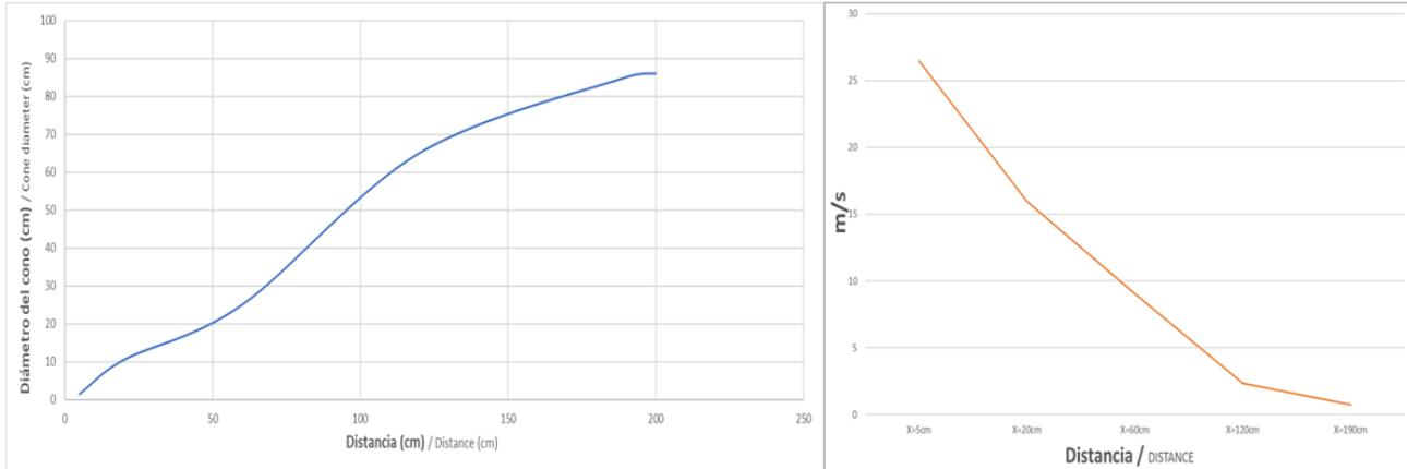
**Figure 5.** (a) Cone diameter with respect to the distance from the end of the nozzle. (b) Velocity in the axis of the cone with respect to the distance from the end of the nozzle.
