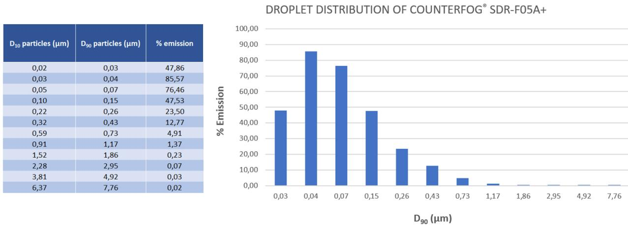
**Figure 6.** Droplet distribution of COUNTERFOG® SDR-F05A+
