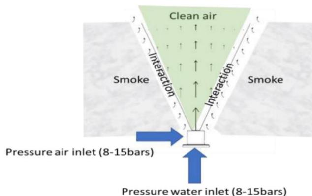
**Figure 2.** Schematic representation of a COUNTERFOG<sup>®</sup> cone absorbing the air -in this case with smoke- around it
