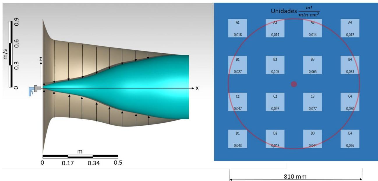
**Figure 4.** (a) Distribution of the airflow drawn in by the fog cone ( $m/s$ ). (b) Distribution of the projected droplets by the fog cone at 2 meters ( $ml/(min \cdot cm^2)$ ).
