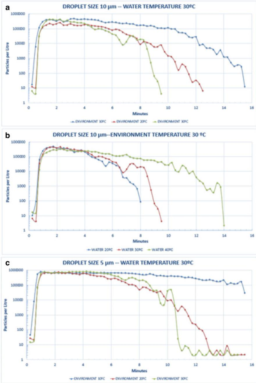
**Fig. 3** (a) Measurement of the colliding time of droplets of 10 μm at different temperatures without COUNTERFOG application. (b) Measurement of the colliding time of droplets of 10 μm at different temperatures with COUNTERFOG application. (c) Measurement of the colliding time of droplets of 5 μm at different temperatures without COUNTERFOG application. (d) Measurement of the colliding time of droplets of 10 μm at different temperatures with COUNTERFOG application
