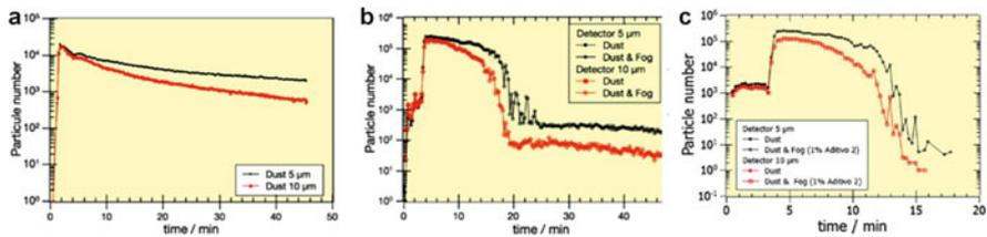
Fig. 3 Comparison of the evolution of different Fog compositions. (a) Talcum dispersed in air and naturally falling down. (b) COUNTERFOG released with just water. (c) COUNTERFOG released with a surfactant additive
